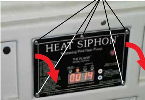
**1** TURN POWER (circuit breaker) OFF and remove the 5 digital door screws. Tilt the door forward until you can access the back of the Player board. Remove the green protective cover from the D-sub connector on the Player board.
